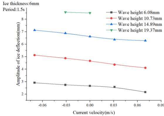
Figure 5 Experimental results of the interaction of wave, current and ice
