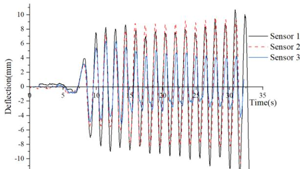
Figure 3 Ice deflection under wave loads
