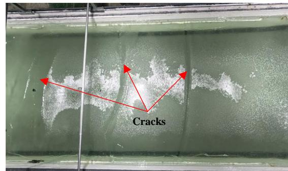
Figure 4 Ice cracks initiation and propagation
