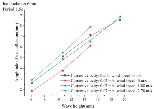
Figure 6 Experimental results of the interaction of wave, wind, current and ice
