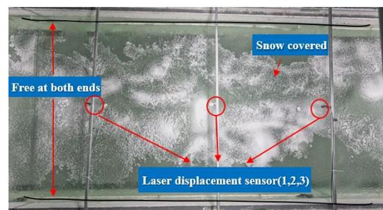
Figure 2 Ice boundary conditions and equipment layout
