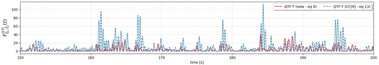
**Figure 3:** Comparison of the time history of the  $x$  component of the second order force  $F_{x, \xi_i \xi_j}^{t7}(t)$ , obtained using the method proposed here (8) and the expression (13) with the upper integration limit being  $t$ .
