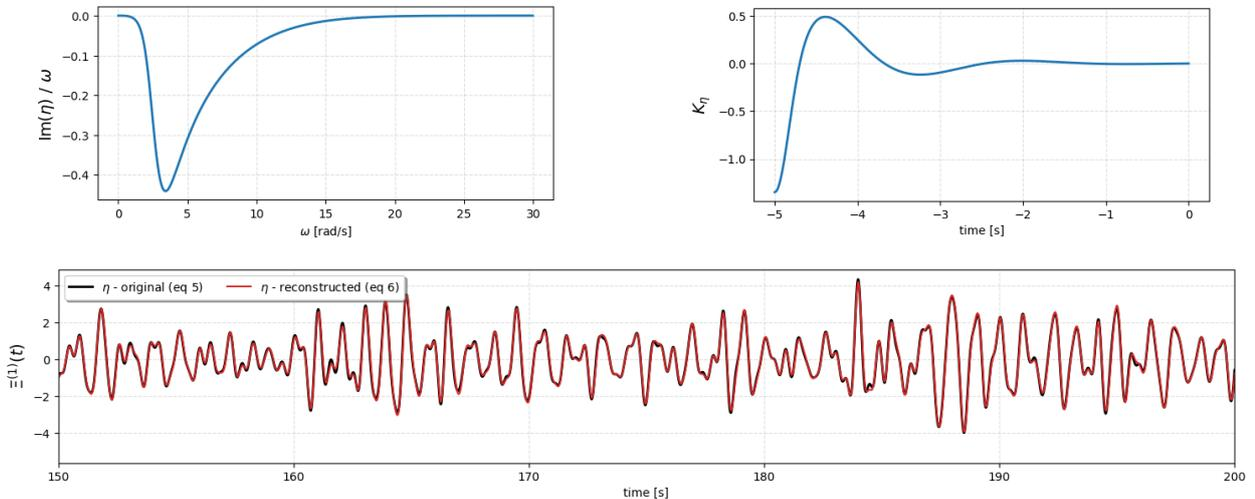
**Figure 1:** Imaginary component of the local wave elevation (left), corresponding memory function (middle) and the comparisons of the reconstructed and the simulated wave elevation, at upstream point, for irregular cylinder motion.
