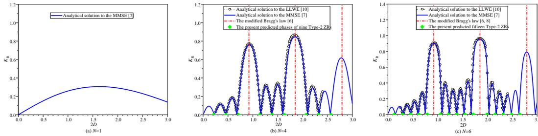
Figure 4: The distribution of ZRs for wave reflection by a trapezoidal bar field with  $h_0 = 2.4$  m,  $B = 0.5$ ,  $w = 8.8$  m,  $w_t = 4.0$  m,  $d = 28.8$  m. (a)  $N = 1$ , (b)  $N = 4$ ; (c)  $N = 6$ .
