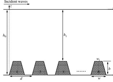
Figure 1: A bar field composed of  $N$  widely spaced periodic trapezoidal bars.
