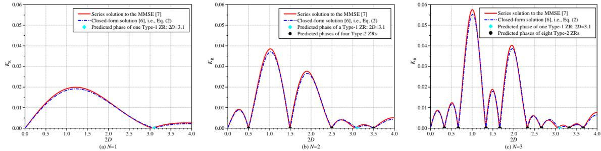
Figure 2: The distribution of ZRs for wave reflection by a trapezoidal bar field with  $h_0 = 0.8$  m,  $B = 0.05$ ,  $w = 1.6$  m,  $w_t = 1.0$  m,  $d = 4.03$  m. (a)  $N = 1$ ; (b)  $N = 2$ ; (c)  $N = 3$ .
