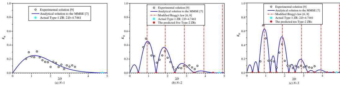
Figure 3: The distribution of Type-2 ZRs for wave reflection by a trapezoidal bar field with  $h_0 = 0.8$  m,  $B = 0.5$ ,  $w = 1.6$  m,  $w_t = 0.4$  m,  $d = 3.6$  m. (a)  $N = 1$ ; (b)  $N = 2$ ; (c)  $N = 3$ .
