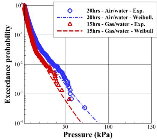
Figure 5: Exceedance probability in low-filling condition: 30% filling, Tank 2, 160K LNG
