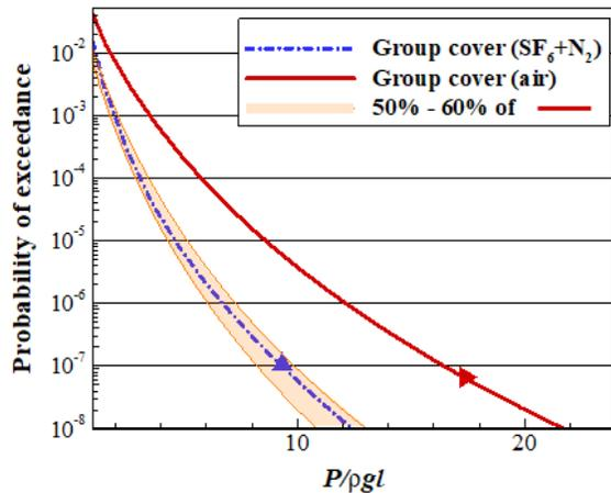
Figure 6: Exceedance probability in high-filling condition: long-term prediction 95% filling, Tank 2, 160K LNGC
