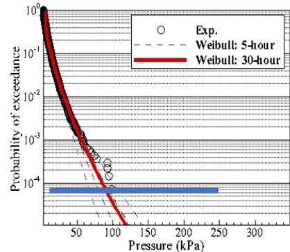
Figure 2: Example of Weibull distribution for short-term prediction
