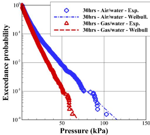
Figure 4: Exceedance probability in low-filling condition: 10% filling, Tank 1, 177K LNGC
