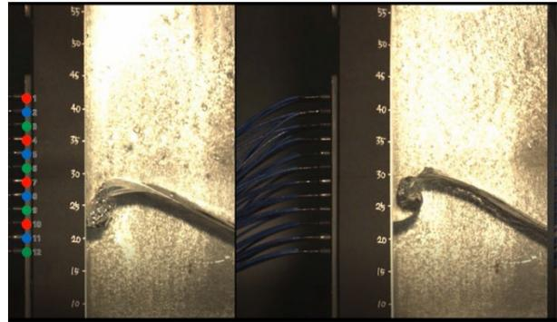
Figure 3: Snapshot of low-filling impact: water-air (left) and water-heavy gas(right) (Lee t al. 2023)
