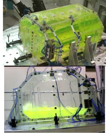
Figure 1: Examples of model-scale sloshing experiment for LNG carrier
