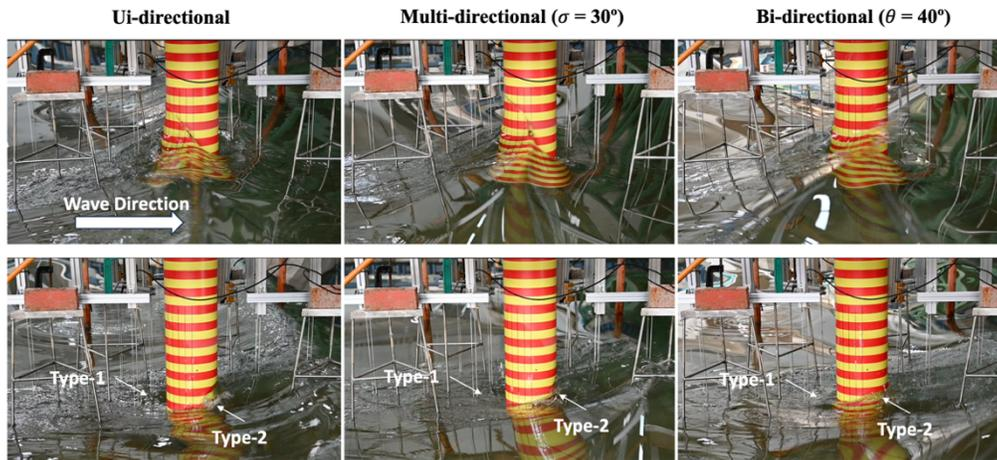
Figure 5: Snapshots from the side view of the cylinder at the time points of (top panel) wave impact and (bottom panel) type-1 and type-2 waves associated with the secondary load cycle.
