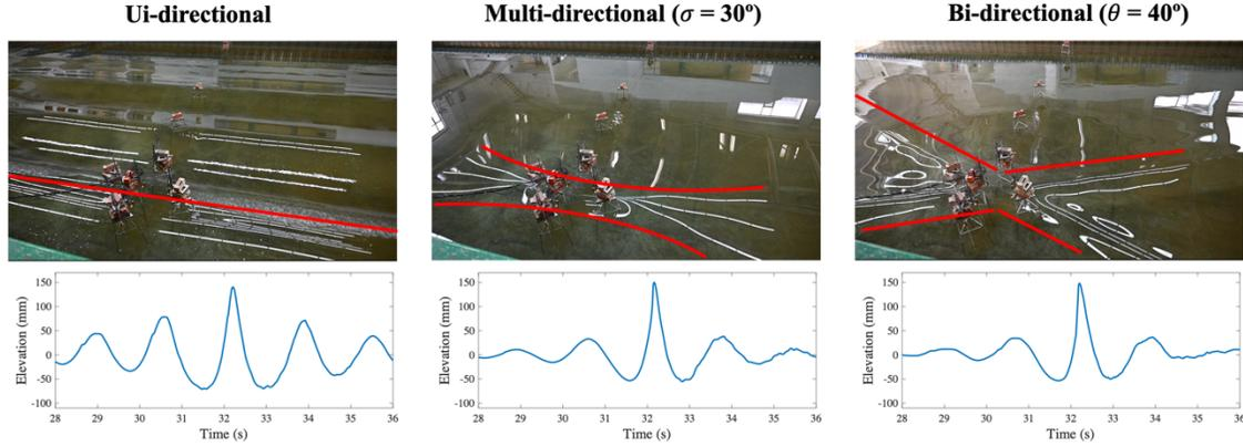
Figure 1: Wave spreading patterns in an empty wave tank and free surface elevation time histories at the focus location under various wave conditions: uni-directional wave ( $T = 1.64$  s,  $A_L = 0.10$  m); multi-directional wave ( $T = 1.64$  s,  $A_L = 0.10$  m,  $\sigma = 30^\circ$ ); bi-directional wave ( $T = 1.64$  s,  $A_L = 0.10$  m,  $\theta = 40^\circ$ ).
