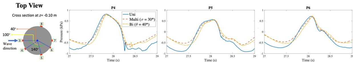
Figure 6: Point pressures measured on the cylinder at 0.10 m below the still water level ( $z = -0.10$  m).
