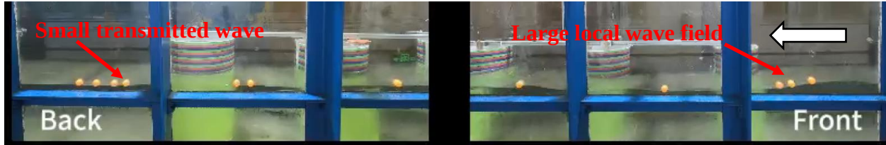
Fig. 3 Photos from the experiments, showing a significant wave energy in front of the cylinder array (right) and a relatively calm water behind the cylinder array (left).
