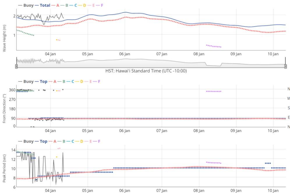
Figure 3. Comparison of records with forecast significant wave heights, peak periods, and directions as well as wave parameters for up to six spectral partitions (A-F) at the Kaneohe buoy.
