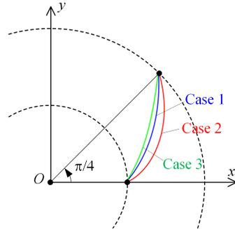
Figure 2: Shapes of the curved plate for the three examined cases with  $R/h = 1.0$ ,  $R_i/R = 0.5$ , and  $\mu(R) = \pi/4$ .
