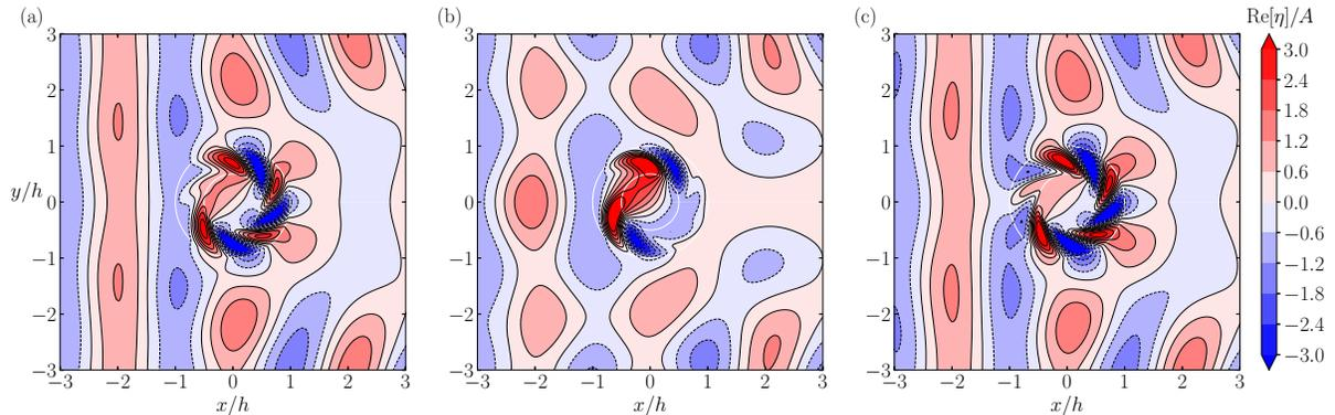
Figure 3: Instantaneous free surface at  $t = 0$  for  $R/h = 1.0$ ,  $R_i/R = 0.5$ ,  $\mu(R) = \pi/4$ , and  $kh = \pi$ : (a) Case 1 ( $a_1 = 0.6617$ ); (b) Case 2 ( $a_2/h = 0.4689$ ); (c) Case 3 ( $a_3\sqrt{h} = 0.7877$ ).
