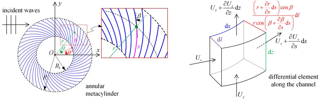
Figure 1: Schematic of an annular metamaterial cylinder consisting of curved plates (left).  $s$  denotes the length of the plate starting from  $(r, \theta) = (R_i, \theta')$  to  $(r, \theta) = (r, \theta' + \mu(r))$ , where  $\mu(r)$  represents the rotation angle of the plate at  $r$ .  $\beta(r)$  denotes the angle of the tangent on the plate relative to the radial direction. A differential element along the channel (right).
