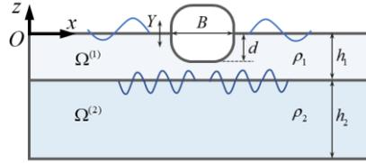
Figure 1: Sketch of two-layer fluids system with an oscillating body
