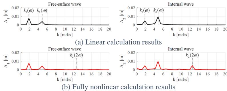
Figure 3: Fast Fourier Transform(FFT) results of wave amplitudes corresponding to wave numbers( $k$ ) [ $KB/2=0.1$ ]
