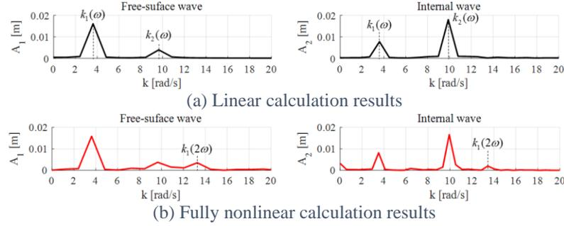
Figure 4: Fast Fourier Transform(FFT) results of wave amplitudes corresponding to wave numbers( $k$ ) [ $KB/2=0.3$ ]
