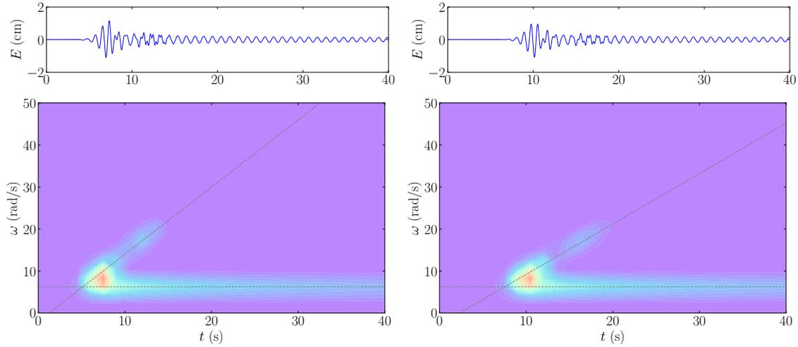
Figure 3: Free surface elevations (top), and the corresponding time-frequency spectrograms (bottom). The measurements at A and B are displayed in the left and right, respectively.
