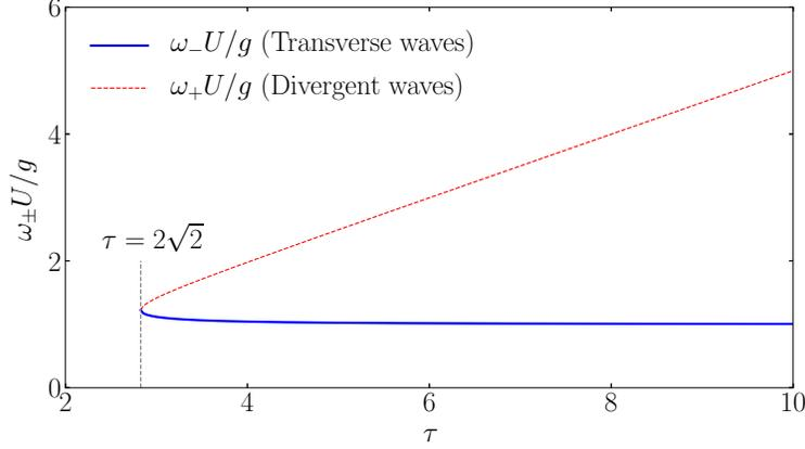
Figure 1: Normalised frequencies of transverse and divergent waves versus  $\tau$ .
