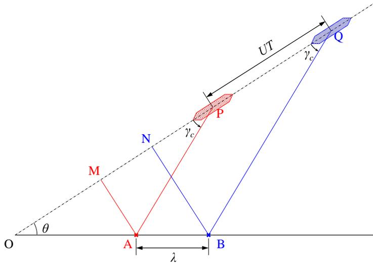
Figure 2: Sketch of a two-probe method to determine ship's speed and sailing direction.
