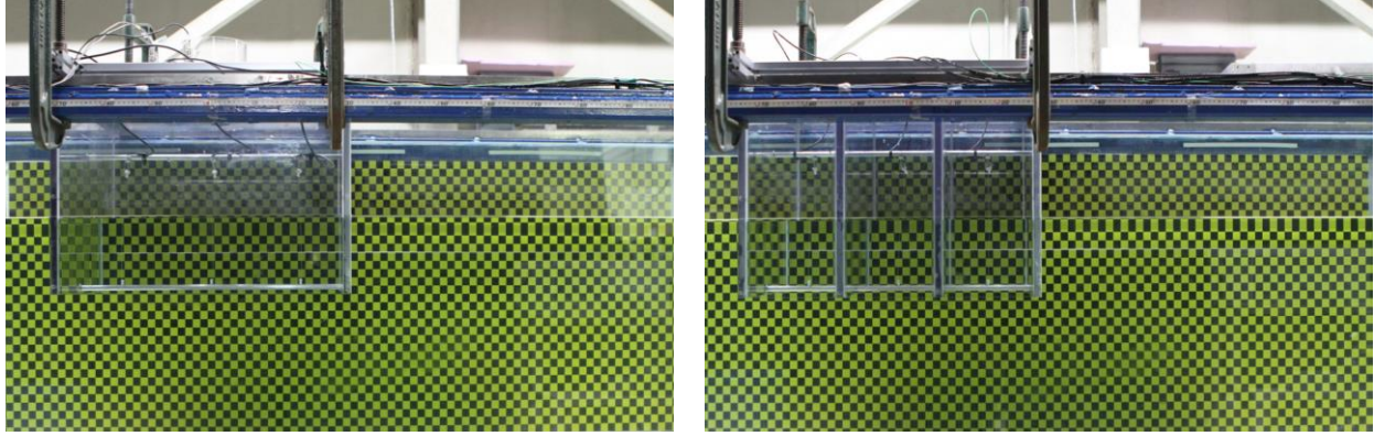
Figure 1: Experimental model of single- and triple-OWC chamber in two-dimensional wave flume
