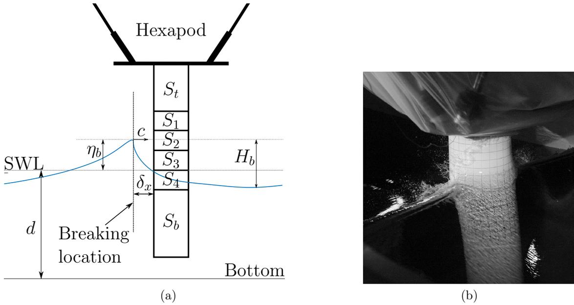
Figure 1: (a) Description of the experimental set-up and (b) picture of a breaking wave impacting the mockup.
