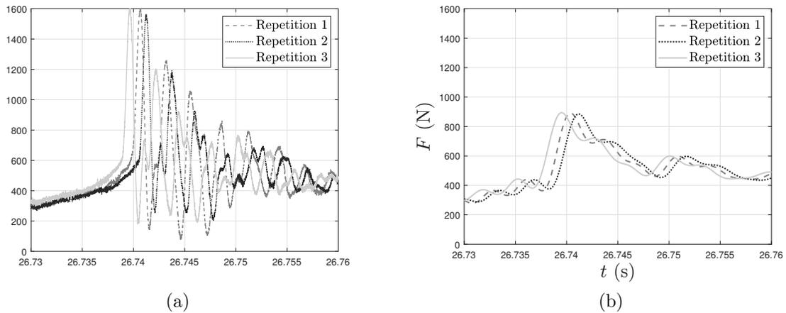
Figure 2: Sum of the (a) raw and (b) 300 Hz low-pass filtered force signal on the four sections along the  $x$ -direction for 3 repetitions of an impact.
