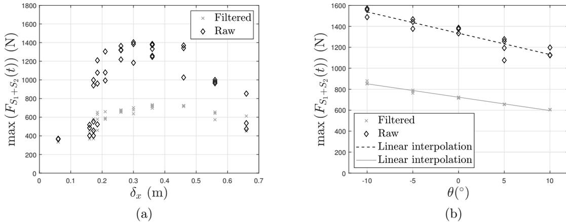
Figure 3: Maximum force measured on the 2 sections during wave impacts (a) at different positions and (b) for different pitch angles.
