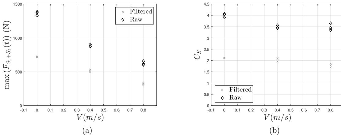
Figure 4: (a) Evolution of the maximum measured force on the two upper sections and (b) of the corresponding slamming coefficient as a function of the mockup horizontal velocity.
