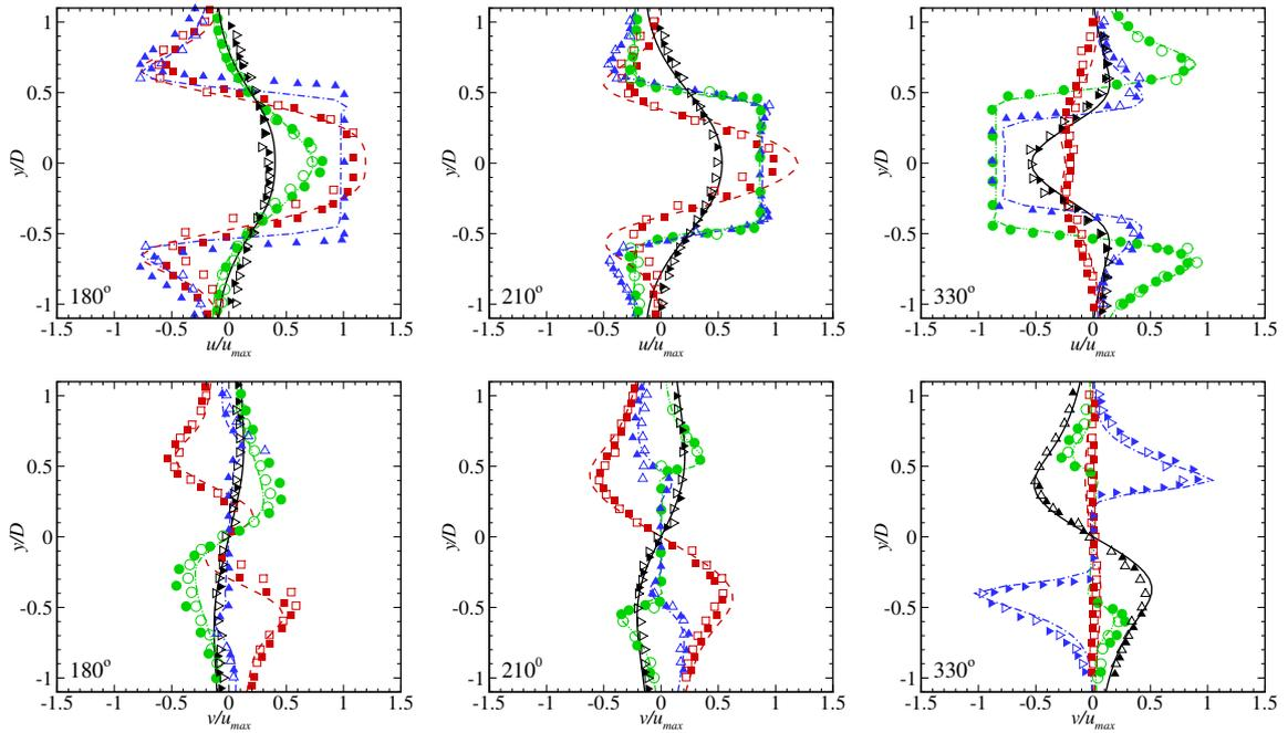
Figure 2: The velocity profiles  $u$  (top) and  $v$  (bottom) at four  $x$  locations in three phases of oscillation:  $x = -0.6D$  ( $- \square \blacksquare$ ),  $x = 0.0D$  ( $- \triangle \blacktriangle$ ),  $x = 0.6D$  ( $- \circ \bullet$ ) and  $x = 1.2D$  ( $- \triangleright \blacktriangleright$ ). The hollow and solid symbols correspond to the numerical and experimental data of [2] and [3], respectively, lines are the current calculations.
