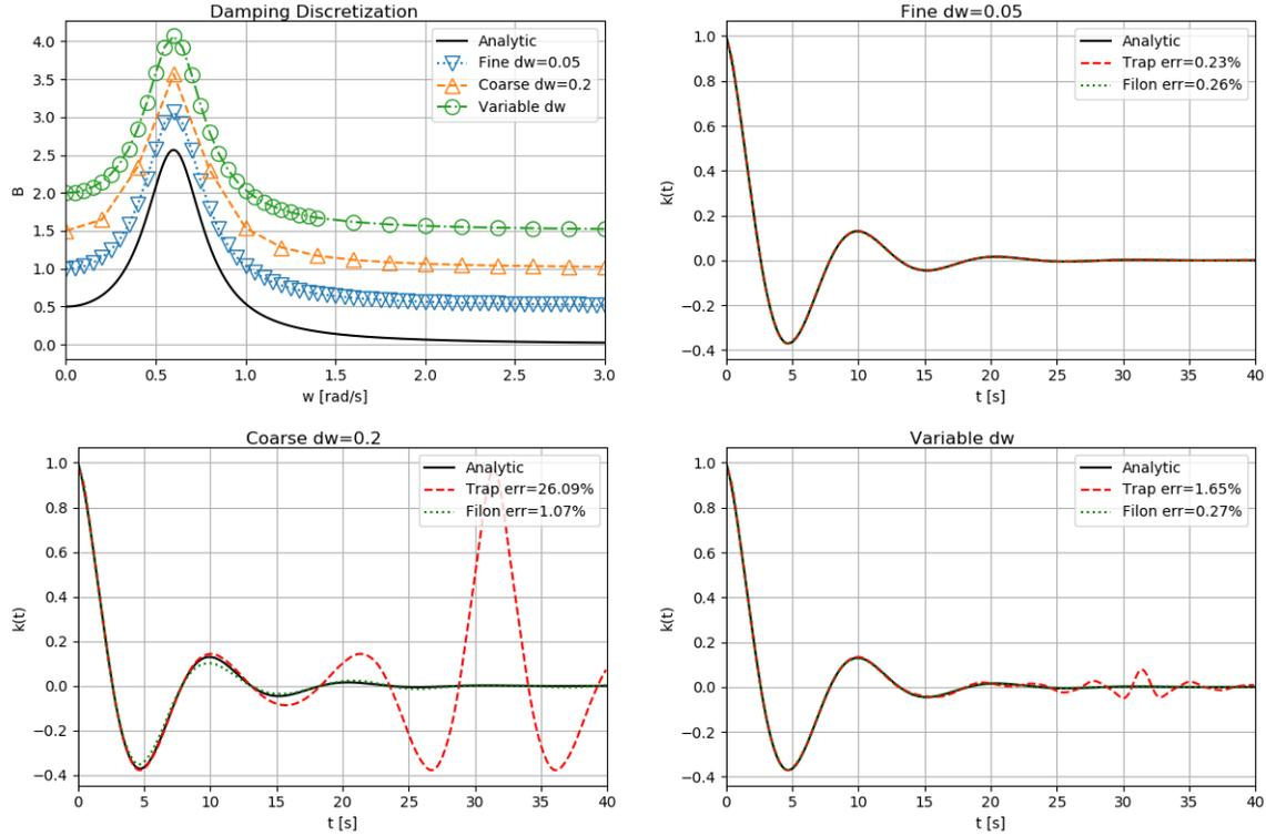
Figure 1: IRF computation with different frequency discretizations
