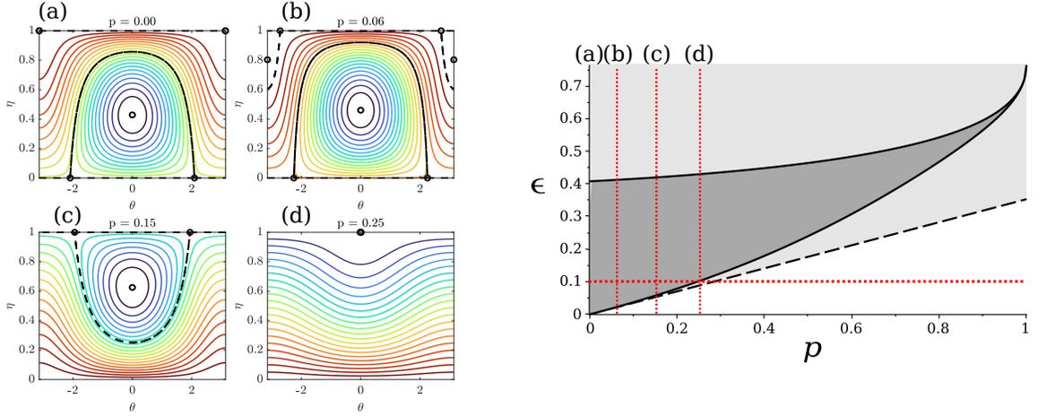
Figure 1: (Left panels) Phase portraits of system (4)–(5) with  $D = 1$  with carrier steepness  $\epsilon_1 = 0.1$  and varying mode separation  $p$ . Dots denote fixed points; thick, dashed lines denote separatrices. (Right panel) Benjamin-Feir instability domains. Dark grey – Zakharov equation. Light grey region – NLS with slope  $\epsilon = p/\sqrt{8}$ . Dotted red lines show  $\epsilon$  and  $p$  for cases (a)–(d) depicted in left panel.
