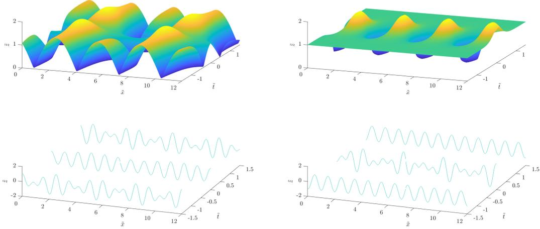
Figure 2: Discrete breather solutions of the BFI system (4)–(5). (Left panels) separatrix connecting fixed points at  $\eta = 0$  (multibreather) showing envelope (top) and free surface (bottom). (Right panels) separatrix connecting fixed points at  $\eta = 1$  (Akhmediev-type breather with plane wave background) showing envelope (top) and free surface (bottom). The  $\tilde{\cdot}$  denotes scaled coordinates.
