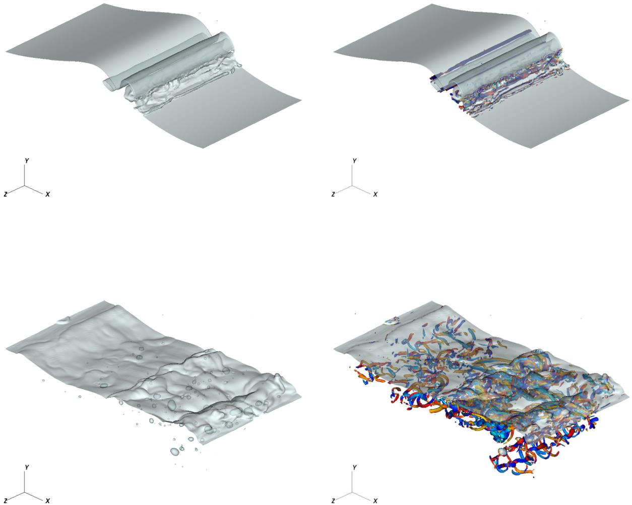
Figure 1: Snapshots of air-water interface (left panel) together with their vortex structures identified by the  $\lambda_2$  method (right panel) at two instants during wave-breaking process.
