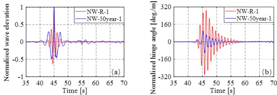
Fig. 4. Examples of transient dynamics effect on this floating hinged raft WEC under wave conditions of NW-R-1 and NW-50year-1. (a) Normalised wave elevation. (b) Normalised hinge angle response.
