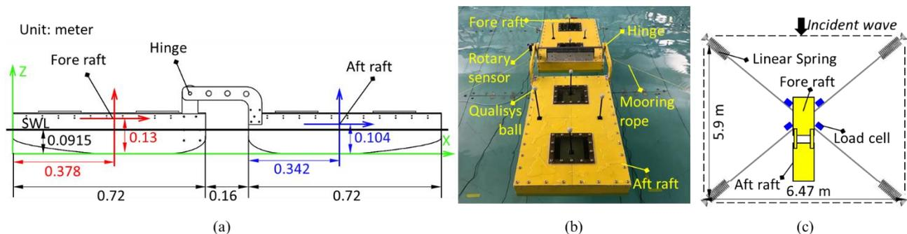
Fig. 1. (a) Dimensions of the designed 1:50 scale hinged raft WEC. The green, red and blue coordinates represent the global coordinate, the centre of gravity (CoG) of the fore raft and the CoG of the aft raft, respectively. (b) Experiment model. (c) Mooring layout.
