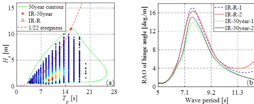
Fig. 2. (a) Schematic of the waves for the EMEC site in full scale. (b) RAOs of the relative hinge angle in full scale.
