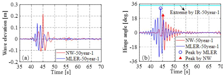
Fig. 5. Comparison of NW and MLER under wave condition of 50year-1. (a) Wave profiles of NW-50year-1 and MLER-50year-1. (b) Hinge angle responses generated.
