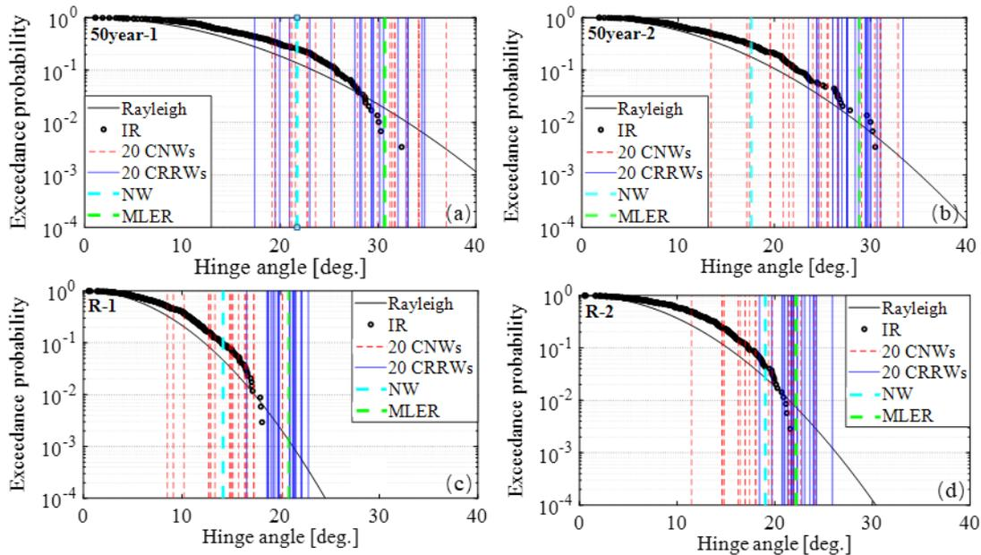
Fig. 6. Comparison of IR, CNW, CRRW, NW and MLER for relative hinge angle response. The theoretical probability distributions are described by the Rayleigh distribution. (a) Under 50year-1. (b) Under 50year-2. (c) Under R-1. (d) Under R-2.
