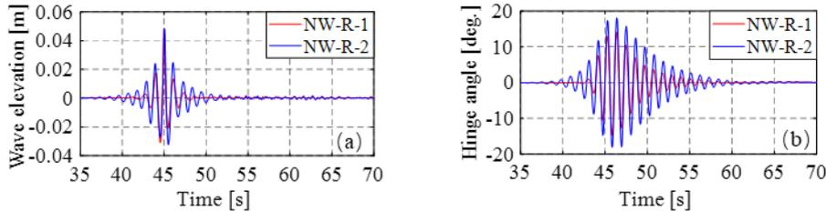
Fig. 3. Examples of proceeding wave effect on this floating hinged raft WEC under wave conditions of NW-R-1 and NW-R-2. (a) Wave elevation. (b) Hinge angle response.
