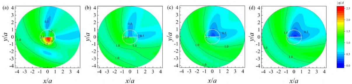
Figure 3: The wave elevation  $h = 2a$  at  $ka = 1$  and  $\beta = \pi/4$  with the damping  $\bar{\gamma} = 0.2$  and spring  $\bar{\kappa} = 0.2$ : (a)  $c/h = 0.25$ ; (b)  $c/h = 0.50$ ; (c)  $c/h = 0.75$ ; (d)  $c/h = 1.00$ .
