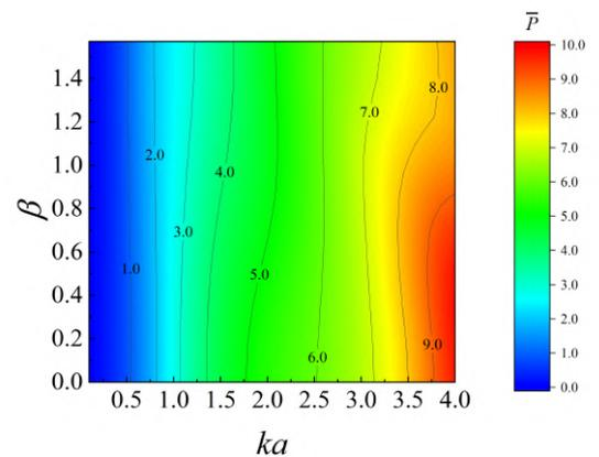
Figure 4: The contour of dimensional wave power generated by the metamaterial cylinder with the paddle length  $c/h = 1$  against the non-dimensional frequency  $ka$  and incident wave angle  $\beta$ .
