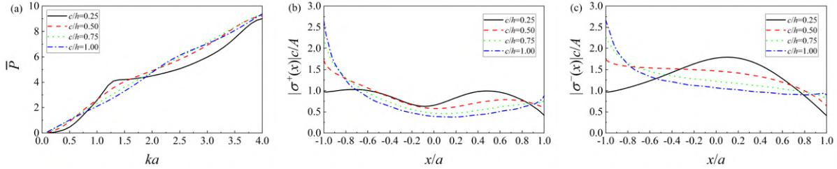
Figure 2: In (a) non-dimensional power generated by the metamaterial cylinder of radius  $a$  in water of depth  $h = 2a$  for an incident wave angle  $\beta = \pi/4$  with dimensionless damping  $\bar{\gamma} = 0.2$  and spring  $\bar{\kappa} = 0.2$ . In (b) and (c) the corresponding amplitudes of the paddle motion at  $ka = 1$ .
