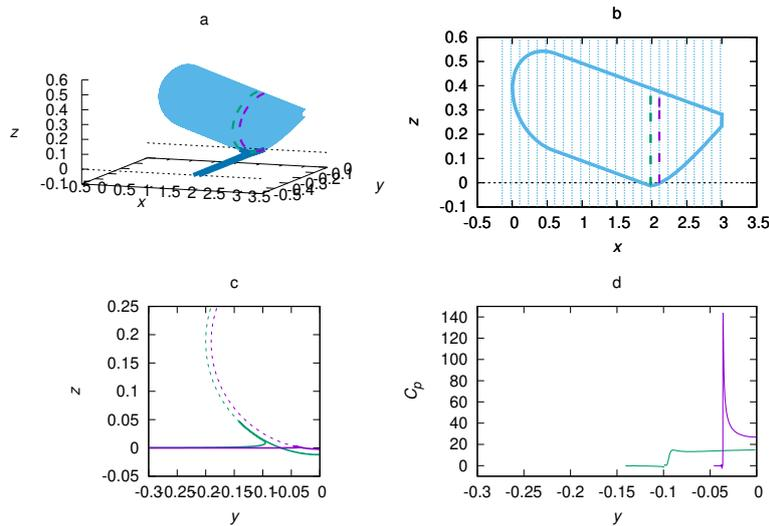
Figure 3: Overview at  $t=0.027s$ . a) 3D view. b) x-z plane: the dashed lines represent the activated sections. c) y-z plane: free surface (continue line) and 2D section (dashed line). d) pressure coefficient distribution acting on the activated sections.
