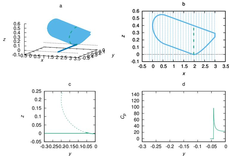
Figure 2: Overview at  $t=0.006s$ . a) 3D view. b) x-z plane: the dashed line represents the activated section. c) y-z plane: free surface (continue line) and 2D section (dashed line). d) pressure coefficient distribution acting on the activated section.
