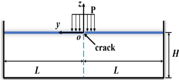
Figure 1. Sketch of a load moving along an ice channel with a crack.
