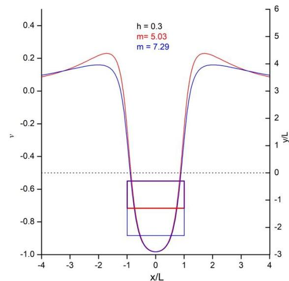
Figure 3. Velocity on the free surface for the square ( $2L \times 2L$ , blue lines), and for the rectangle ( $2L \times L$ , red lines).
