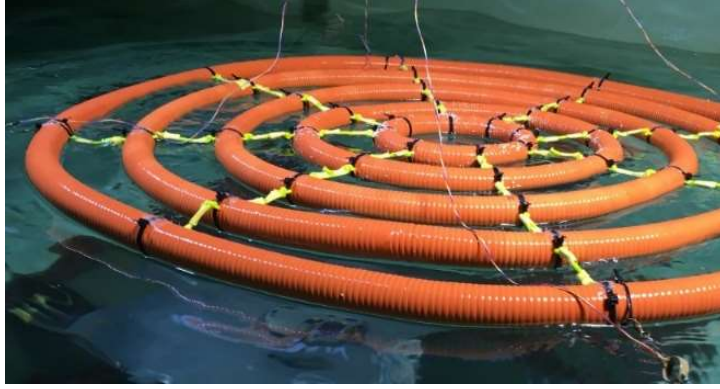
Figure 1. Multi-torus solar island model. Left: Preliminary experiments at NTNU 2018 and 2019. 2R_1 = 1\text{m} . Cross-sectional diameter 2c = 0.032\text{m} . Torus axis-to-axis distance 2p = 0.05\text{m} . EI = 0.847\text{Nm}^2 . Right: Sketch with parameter explanations. The coordinate system is right-handed, such that the z -axis is positive upwards, and the origin is at the still water level. Waves travel along the positive x -axis.
