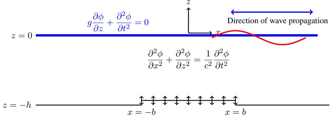
Figure 1: Schematic diagram of the physical problem. The ocean bottom in  $-b < x < b$  is oscillating vertically.
