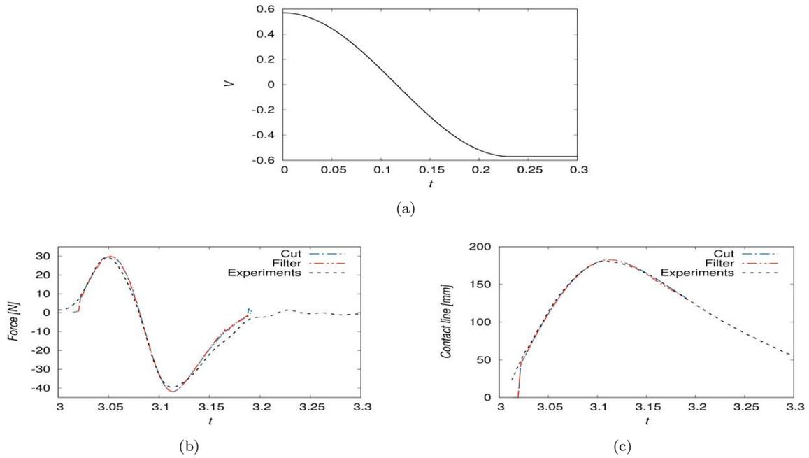
Figure 6: Velocity (positive downward) (a), non dimensional force (b) and contact line (c) distribution for the cone case
