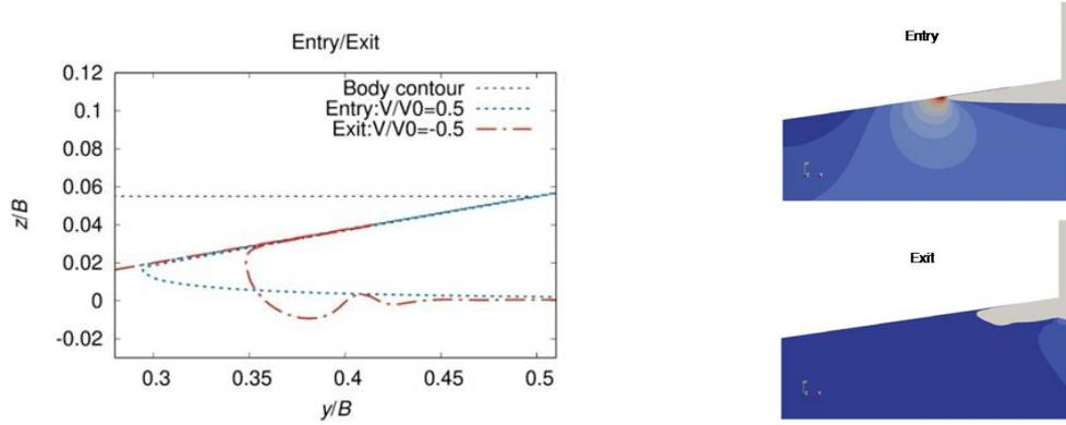
Figure 3: Wetted length during entry and exit phase. On the right there are CFD results [6]
