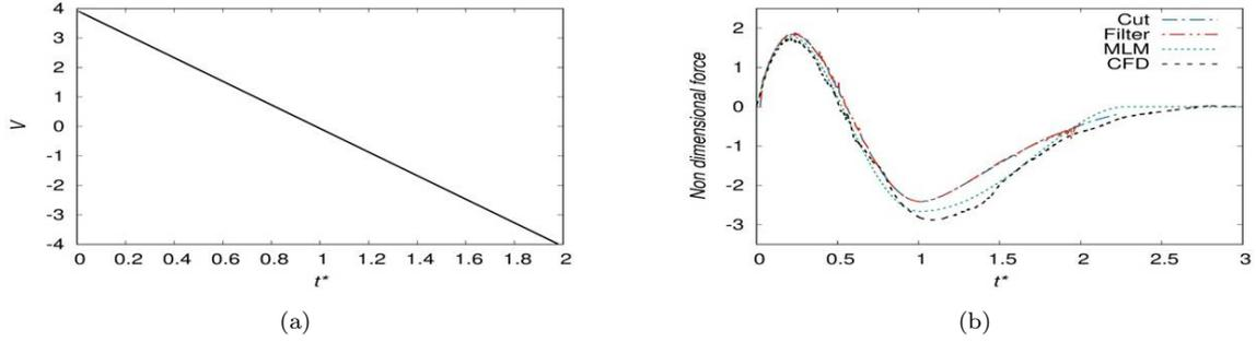
Figure 5: Velocity (positive downward) (a) and non dimensional force (b) distribution for the wedge case
