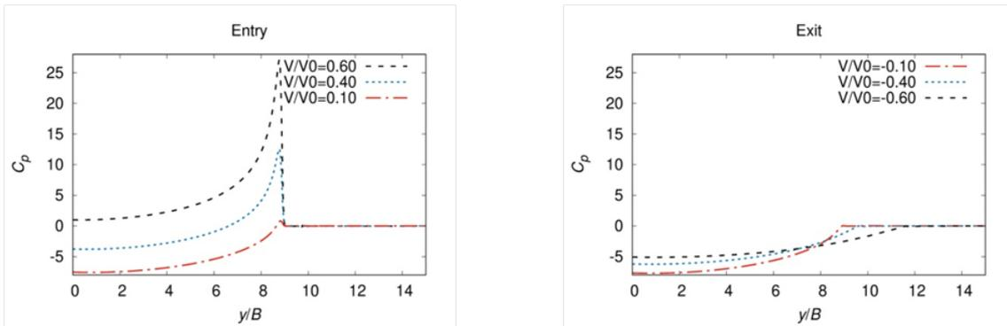
Figure 4: Pressure coefficient distribution
