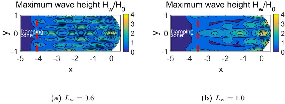
**Fig. 3.** Spatial distribution of the maximum wave height of reflected wave field, for (a)  $L_w = 0.6$ ; (b)  $L_w = 1.0$
