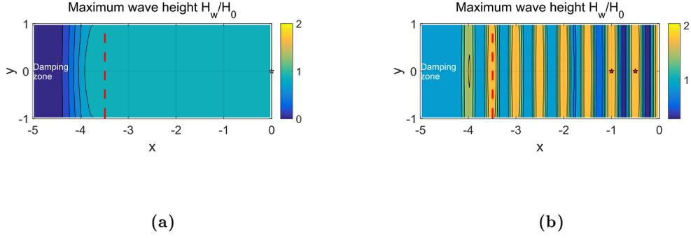
**Fig. 2.** Spatial distribution of the maximum wave height of (a) reflected wave field; (b) full wave field
