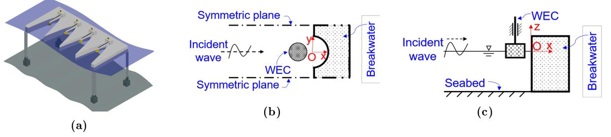
**Fig. 1.** Model of a parabolic OB-WEC breakwater: (c) design example; (b) top view; (c) side view
