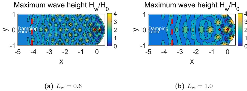
**Fig. 4.** Spatial distribution of the maximum wave height of full wave field, for (a)  $L_w = 0.6$ ; (b)  $L_w = 1.0$
