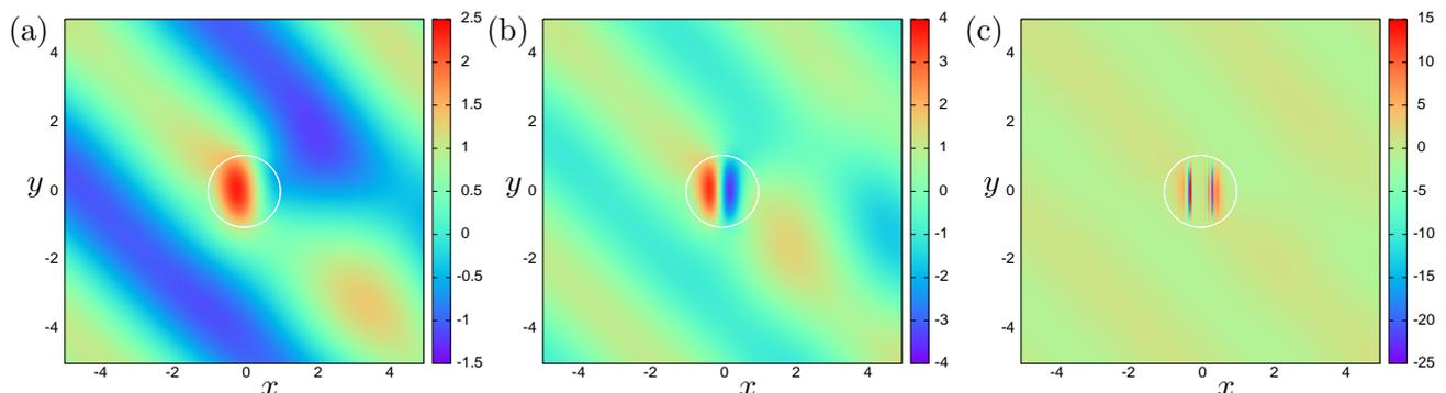
Figure 3: Instantaneous wave field due to incident wave propagating with  $\theta_0 = 45^\circ$  on a cylinder with  $a = 1$  with: (a)  $k = 1$ ; (b)  $k = 1.3$ ; (c)  $k = 1.6$ .
