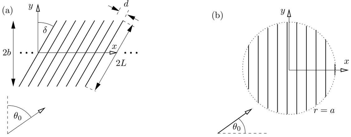
Figure 1: (a) A parallel-plate array metamaterial of finite width and (b) a circular parallel-plate array metamaterial cylinder.
