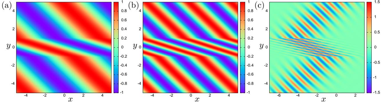
Figure 2: The instantaneous wave field for incident waves propagating at  $\theta_0 = 45^\circ$  into an array of plates tilted at  $\delta = -45^\circ$  for  $k = 1$  (a) and  $k = 2$  (b). In (c) a Gaussian beam is incident at  $kL/2\pi = 9$ .
