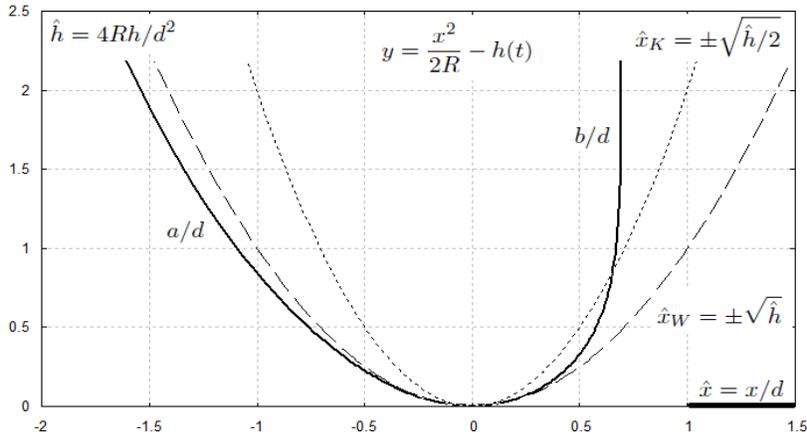
**Fig. 3** The coordinates of the contact points calculated by different models.
