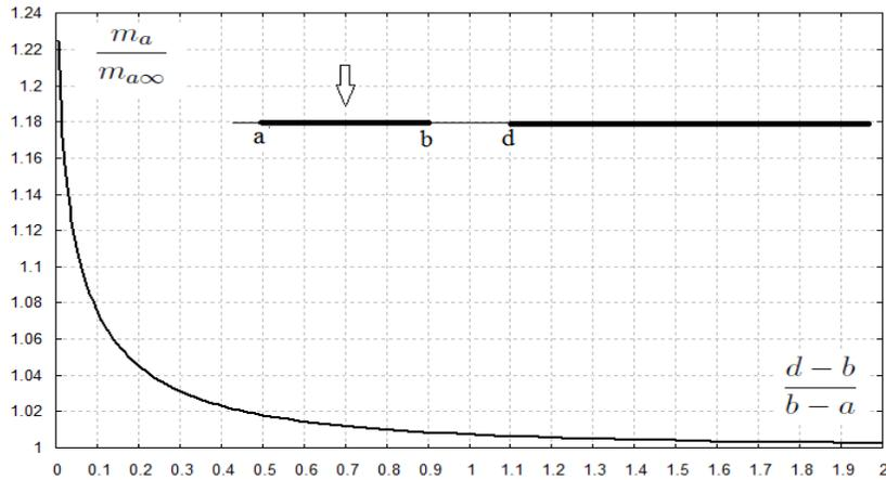
**Fig. 2**  $M_a$  as a function of the relative gap length between the impacting plate ( $a, b$ ) and the semi-infinite ice sheet ( $d, \infty$ ).
