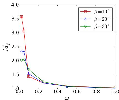
**Fig. 4**  $M_f$  as a function of the relative gap length  $\omega$  between the impacting body and the semi-infinite ice sheet.
