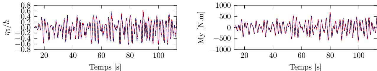
FIGURE 8 – ART with bathtub vortex : Comparison between an irregular roll motion and its equivalent irregular sway motion (dotted blue line). (At left) Time series of the free surface elevation at  $x/L = 0.475$  (At right) moment  $M_x$ .
