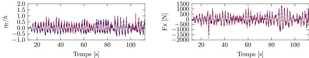
FIGURE 7 – Rectangular ART : Comparison between a 6DOF irregular motion and its equivalent irregular pure roll motion (dotted blue line). (At left) Time series of the free surface elevation at  $x/L = -0.375$  (At right) force  $F_y$ .
