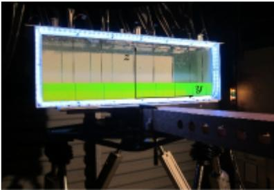
FIGURE 4 – Experimental set-up. Tank mounted on the Hexapod
