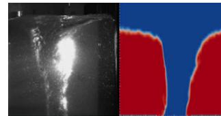
FIGURE 2 – Experimental and numerical bathtub vortex
