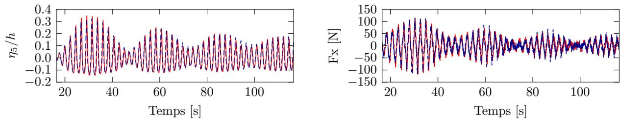
FIGURE 6 – Rectangular ART : Comparison between the pure sinusoidal roll motion of amplitude  $R_x = 0.5\text{deg}$  (red line) and its equivalent pure sinusoidal sway motion of amplitude  $T_y = 10.902\text{mm}$  (dotted blue line) at  $f/f_1 = 1.121$ . (At left) Time series of the free surface elevation at  $x/L = 0.475$  (At right) force  $F_y$ . A nonlinear beating as described in Faltinsen [9] is observed.
