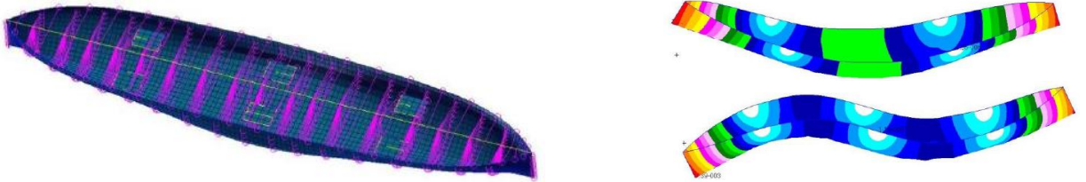
Fig. 1 Structural model and the first two vertical bending modes for the modified Wigley model
