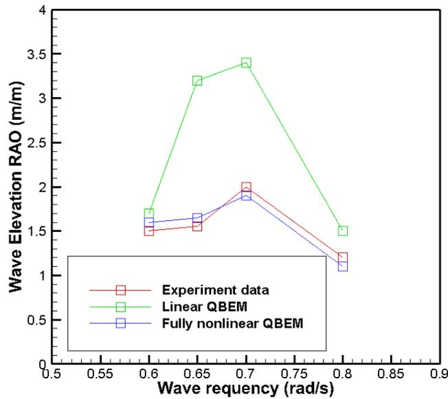
Fig. 3. Comparison of total wave elevation RAO (at the center of the gap) in the neighborhood of the resonance frequency among the linear and fully-nonlinear simulations as well as experimental data. Fully-nonlinear solution compares excellently with the experimental data. (Gap width = 32m,  $kA=0.05$ , head sea, diffraction problem).
