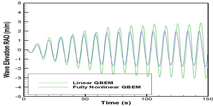
Fig. 2. Time history of the total wave elevation at the center of the gap between two ships obtained from linear and fully-nonlinear simulations. (Gap width = 32m, incident wave steepness  $kA=0.05$ , head sea, diffraction problem).
