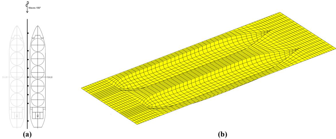
Fig. 1. (a) Configuration of two ships in the experimental setup, and (b) sample QBEM computational grids.
