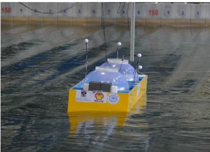
Fig. 1 The horizontally moored model in the wave basin.
