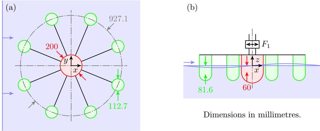
Figure 1: The configuration of the cloaking apparatus: (a) plan view, (b) side view.
