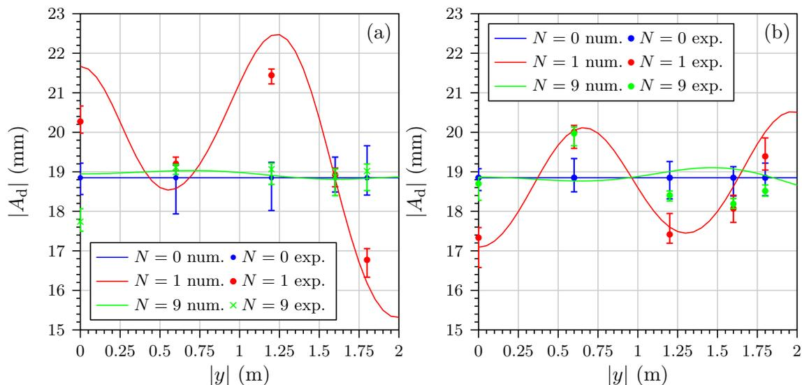
Figure 4: Diffraction wave amplitude with  $N$  cylinders installed: (a) 2 m upwave (gauges 3-7), (b) 2 m downwave (gauges 9-13).
