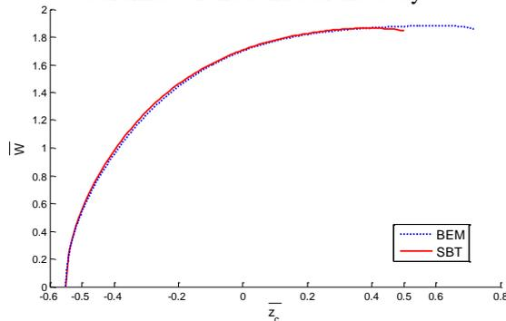
Fig. 4. Velocity of the body versus the vertical coordinate of the centre of the body
