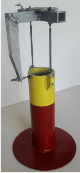
Figure 1: Column with a circular heave plate attached to a frame
