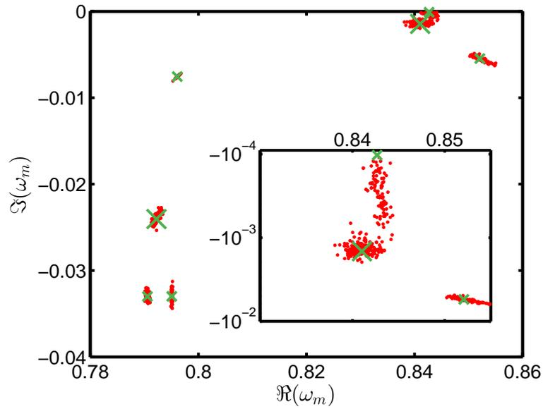
Figure 5: The case of nine cylinders with water depth  $h = 4$  and draft 1. The crosses show the positions of the resonances as in figure 3 while the dots show configurations in which the cylinders are slightly perturbed from this mean position
