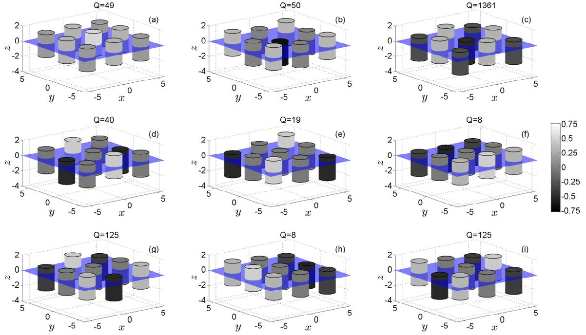
Figure 4: The real part of the nine complex resonance vectors for the nine cylinder array.
