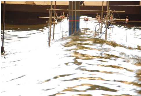
Figure 1: Left: Wave incident at a vertical cylinder. Right definition sketch for the diffraction problem with a large domain for incident wave computation and a smaller flat-bed domain for the diffraction computation.
