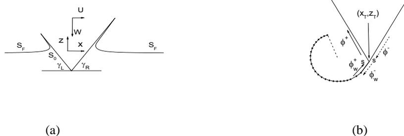
Fig.1 illustration of (a) the wedge water entry with vortex shedding and (b) the local wake surface
