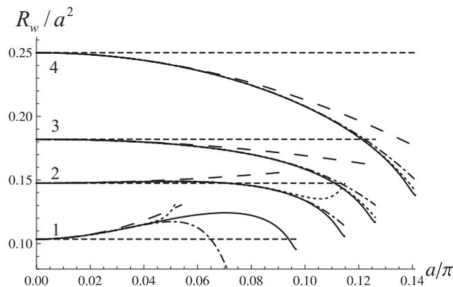
Figure 3: Comparison of accurate numerical results with analytical formulae at the depths  $\frac{d}{2\pi} = 0.15$  (1), 0.2 (2), 0.25 (3)  $\infty$  (4): solid lines, the waves have been computed by the method of the paper by Maklakov (2002); dashed lines,  $n = 1$  (Kelvin's one-termed formula), dashed lines with long dashes,  $n = 2$ ; dot-and-dash lines,  $n = 5$ ; dotted lines,  $n = 10$ , where  $n$  is the number of terms in (20).
