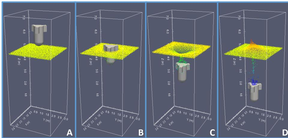
Figure 4: Snapshots of numerical simulation for solid impacting free surface. The colour represents the height of free surface particle position; the warmer colour means the higher position.
