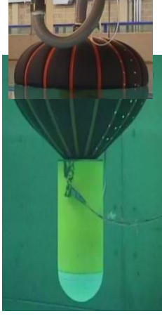
Figure 2. Combined under- and above-water images of the bag and ballast container.
