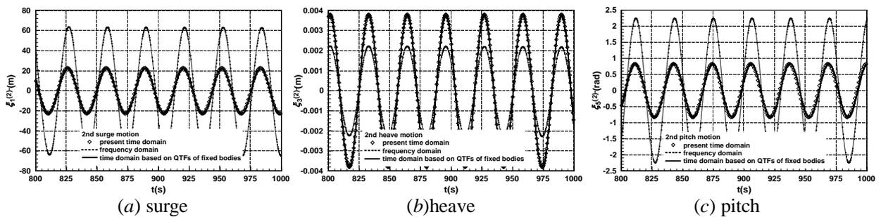
Fig.2 Second-order difference frequency body motion results.
