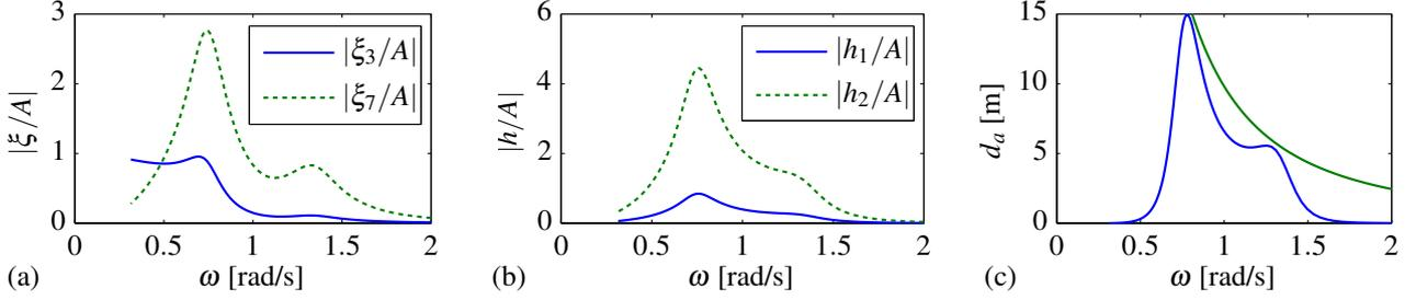
Figure 4: Numerical results for the floating device as shown in Fig. 2: (a) displacements, per unit incident wave amplitude, of the float and of the moving surface relative to the float, for  $F = 0.003$  ms; (b) corresponding displacements, per unit incident wave amplitude, of the water column levels relative to the float; (c) corresponding absorption width, compared to the theoretical limit  $\lambda/2\pi$  (descending line).
