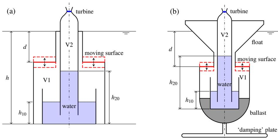
Figure 1: Sketch of the (a) bottom-fixed and (b) floating devices. The moving surface is free to move up and down. The sketch is representative only and not intended as a practical design.
