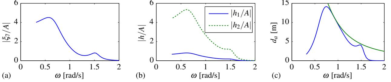
Figure 3: Numerical results for the bottom-fixed device as shown in Fig. 2: (a) displacement, per unit incident wave amplitude, of the moving surface, for  $F = 0.0015$  ms; (b) corresponding displacements, per unit incident wave amplitude, of the water column levels; (c) corresponding absorption width, compared to the theoretical limit  $\lambda/2\pi$  (descending line).
