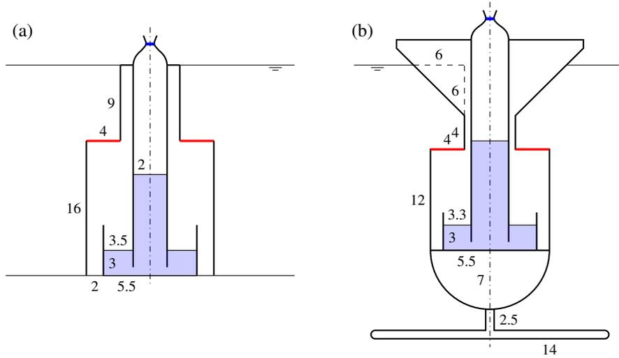
Figure 2: Dimensions (in m) of the (a) bottom-fixed and (b) floating devices. The total displaced volume of the bottom-fixed device is  $3174 \text{ m}^3$ , and  $V_{10} = 2612 \text{ m}^3$ . The total displaced volume of the floating device, neglecting the ‘damping’ plate, is  $3414 \text{ m}^3$ , and  $V_{10} = 3086 \text{ m}^3$ . The water depth is assumed to be infinite for the floating device case.
