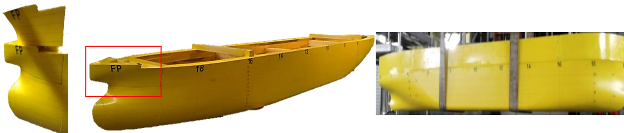
(a) Original (above) and Ax-bow (below) of KVLCC2 (b) Modified KVLCC2 with leage bow Fig. 3 Hull forms of KVLCC2 tanker with three different bow shapes
