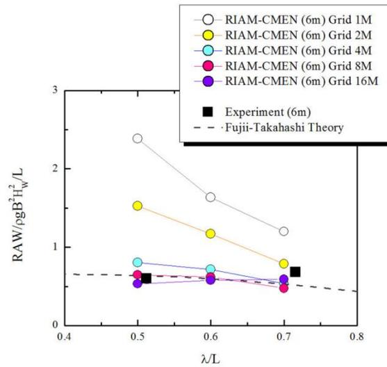
Fig.2 Grid convergence test on added resistance
