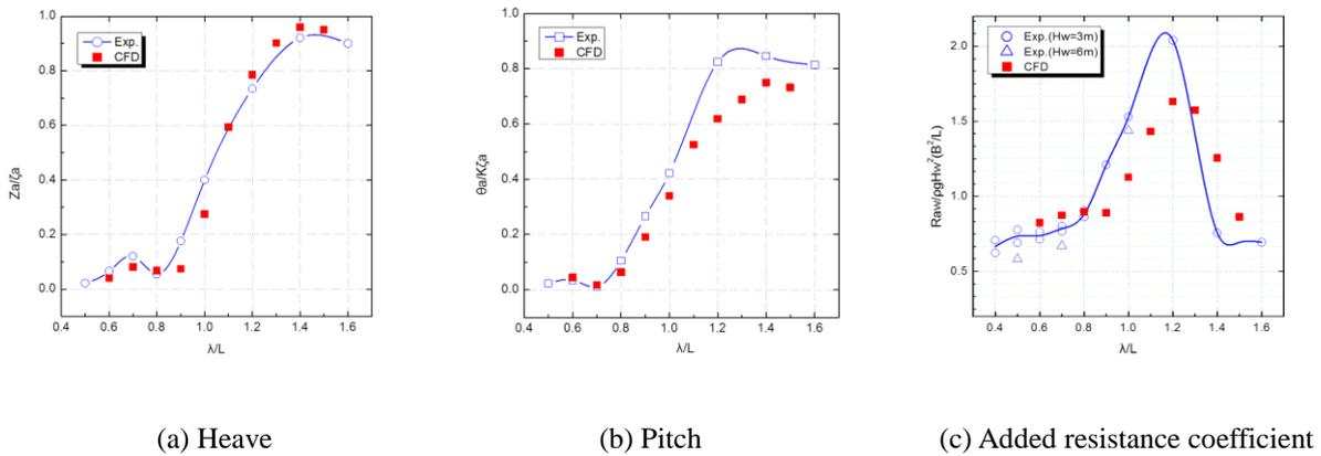
Fig.3 Comparison of RAOs between experiment and CFD
