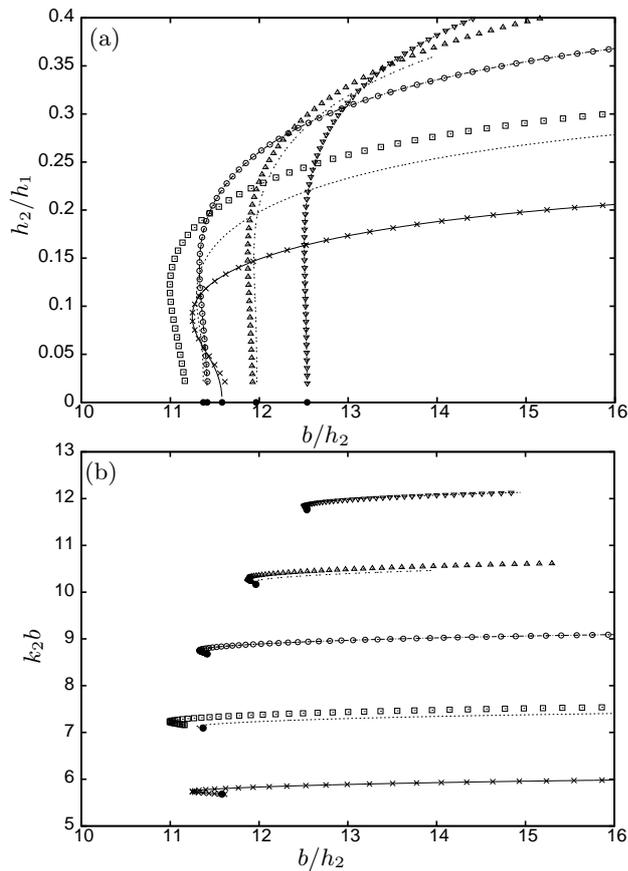
Figure 2: Parameter variations for transparency of a submerged plate. Lines and symbols show exact and wide-spacing results.
