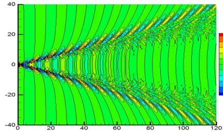
Figure 4: Contours of the wave elevation with  $\sigma = 0.2, \varepsilon = 1.0e - 7, z_0 = 0.4$ .
