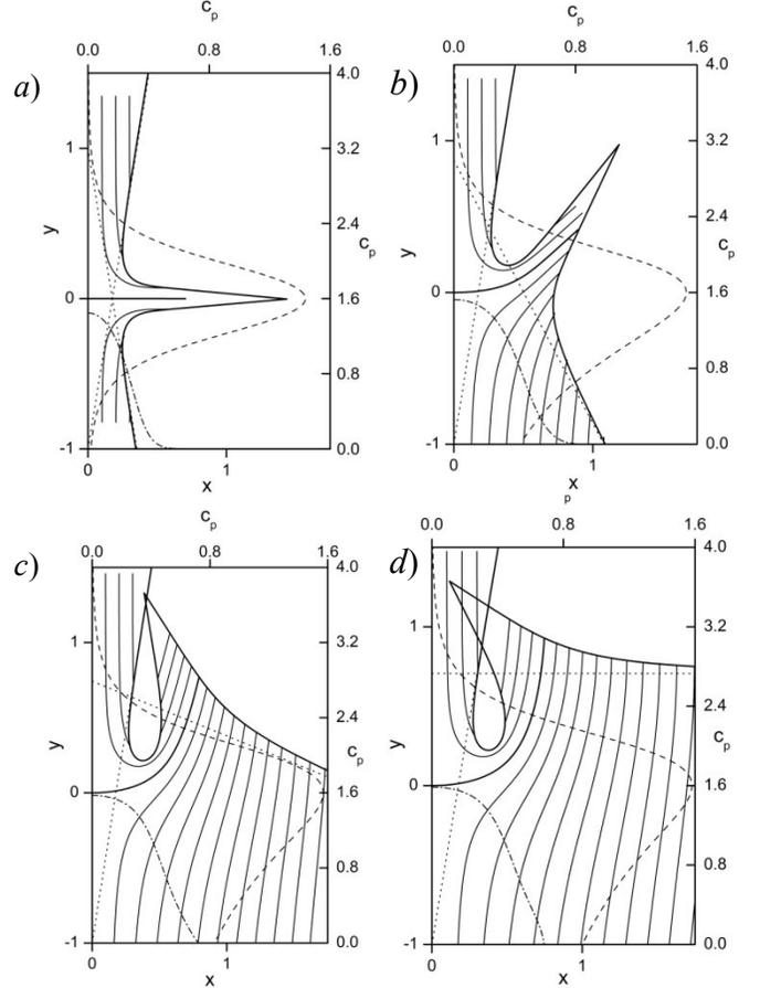
Figure 2. Streamline patterns (solid lines) and the pressure distribution along the  $y$ -axis (dashed line) and along the "zero" streamline starting at the origin (dot-dashed lines) for  $\alpha_+ = 10^\circ$  and (a)  $\alpha_- = 10^\circ$ , (b)  $30^\circ$ , (c)  $70^\circ$  and (d)  $90^\circ$ . Here,  $c_p = c_p^* - c_{pO}^*$ , where  $c_{pO}^*$  is the pressure coefficient at point  $O$  or at any point on the free surface.
