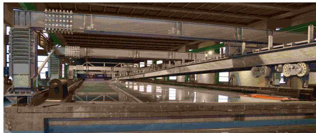
Figure 1: View of the CNR-INSEAN guided ditching facility. The guide is supported by bridges which can be varied in height in order to get the correct U/V velocity ratio. The main trolley can be also seen on the right.
