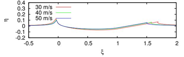
Figure 5: Free surface shapes obtained for a plate incidence  $\gamma = 10$  at different horizontal velocities. For the sake of the clarity, on the right hand side of the plate, the thinnest part of the jet, described by the shallow water model, is not depicted.
