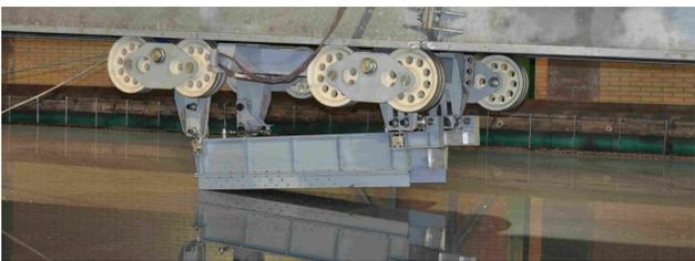
Figure 3: Picture of the trolley with model at the touch of the free surface. Note that the specimens is not installed yet.
