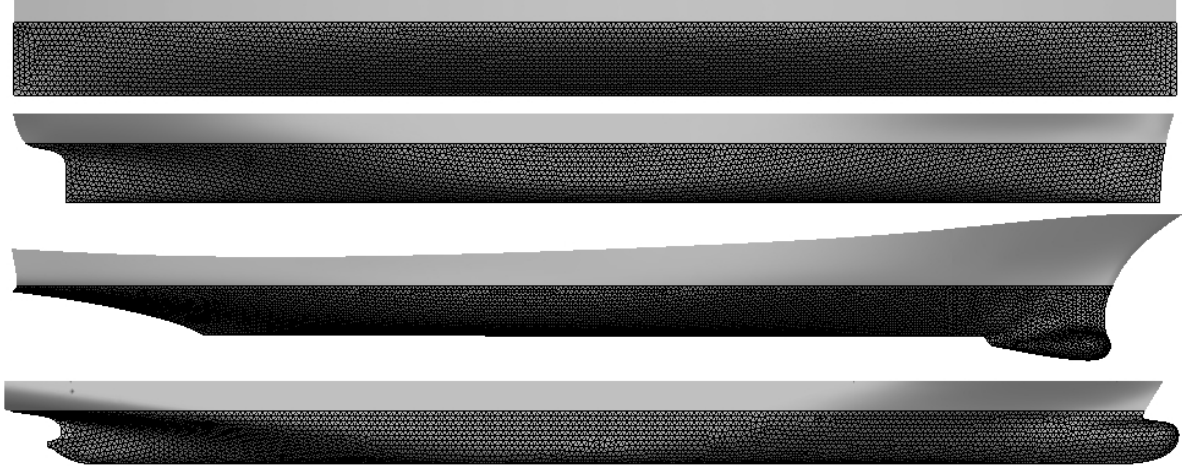
Figure 3: Side views, with meshes over the mean wetted hull surfaces, of the Wigley hull (top row), the Series 60 C_b = 0.60 model (second row), the DTMB-5415 model (third row) and the KCS model (bottom row). The positive halves of these four hull surfaces are approximated using 8,000 flat triangular panels for the Wigley hull and the Series 60 model, 9,600 panels for the DTMB-5415 model, and 18,960 panels for the KCS model (fewer panels are shown in the figure for clarity).
