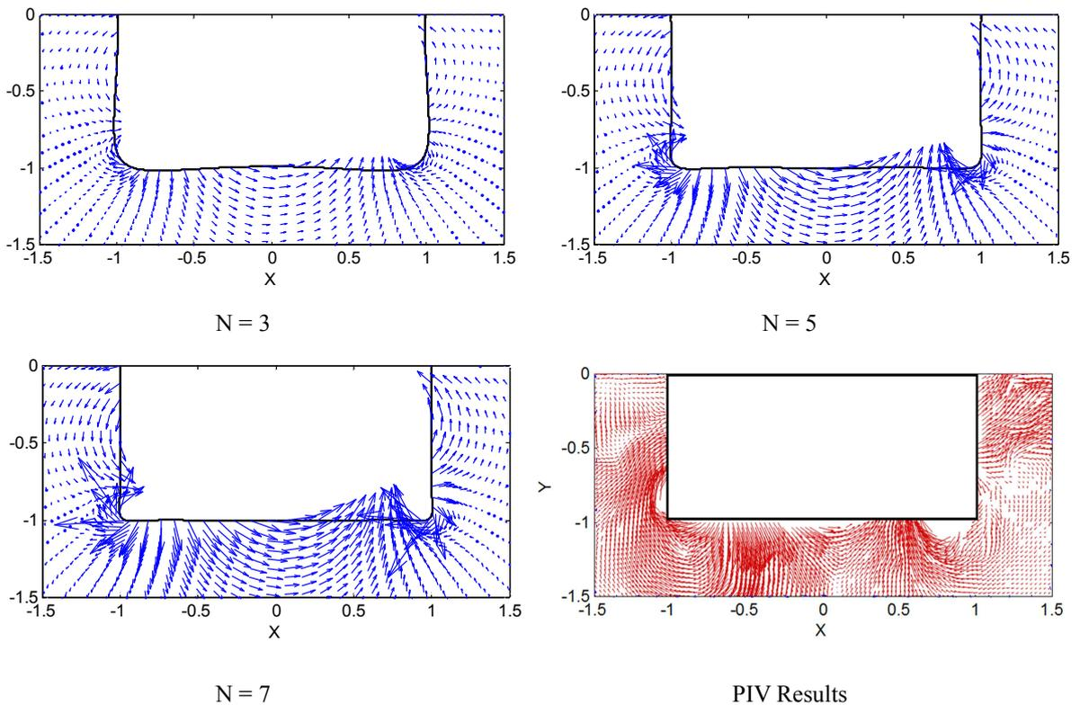
Fig. 7 Computed Flow Fields Compared to PIV Result
