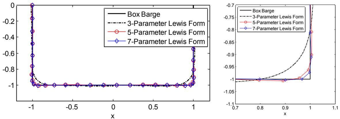
Fig. 1 Hull Form for Various Number of Parameters
